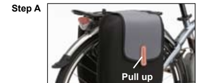
Power Control Switch - Two EnergyPak Hybrid bicycle Turn to "Off" to remove EnergyPaks
