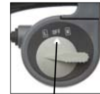
Power Control Switch - Two EnergyPak Hybrid bicycle Turn to "Off" to remove EnergyPaks
