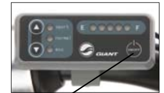
RideControl Command Center - Single EnergyPak Hybrid bicycle Push "ON/OFF" button to "OFF" to remove EnergyPak
