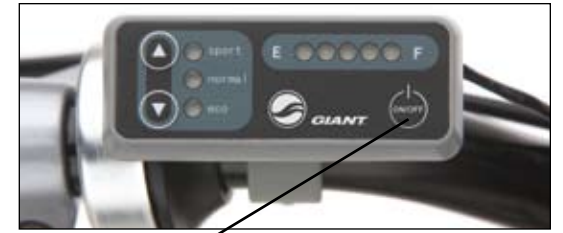
RideControl Command Center – Single EnergyPak model Push "ON/OFF" to activate Hybrid Power
