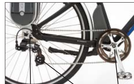
Chainstay dropout and PedalPlus Power Sensor Rear derailleur Crankset
